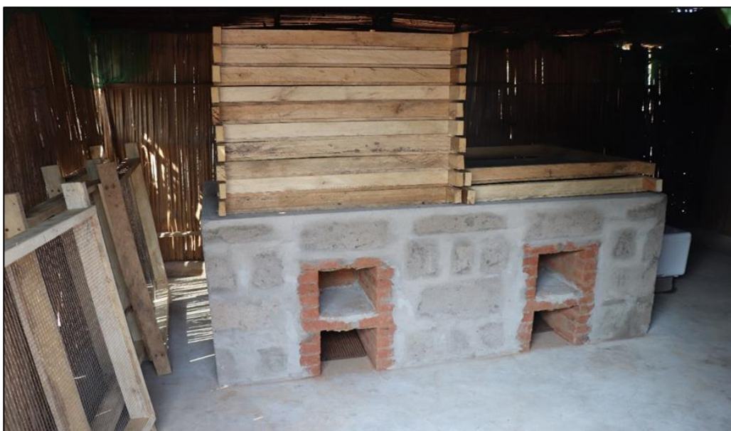
Figure 2 Ahotor Oven with layered fish smoking racks BAP: 2, PAH4: 10.93 \mu g/kg, Price: $400 (GHS 2,500)
