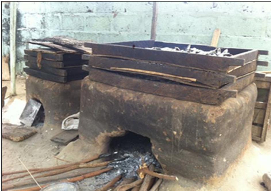
Figure 18. The Chorkor smoker, which is being replaced with the more environmentally-friendly Ahotor oven.
