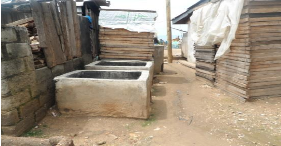
Plate 6 A sample of good Chorkor Ovens in Winneba community – fish processing site
