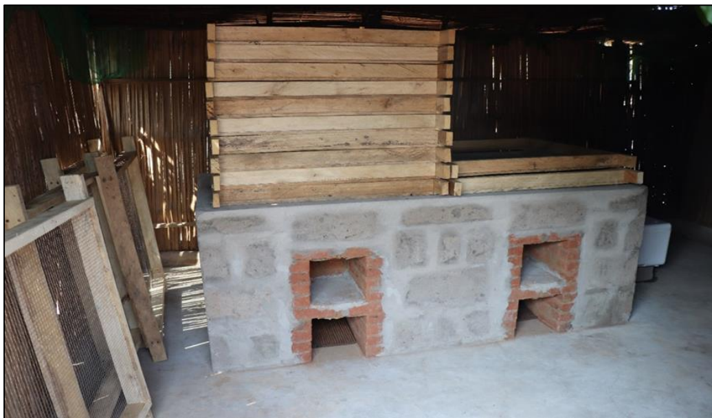
Figure 4. Ahotor Oven with layered fish smoking racks
