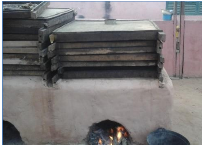
Figure 9 Drying process with a plywood cover
