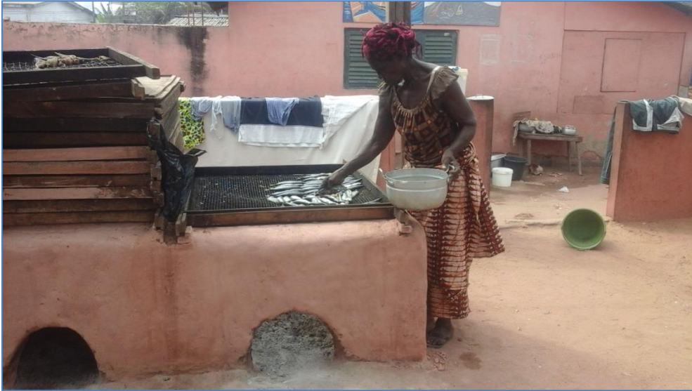
Figure 6 Arranging fish on the tray of a Morrison stove
