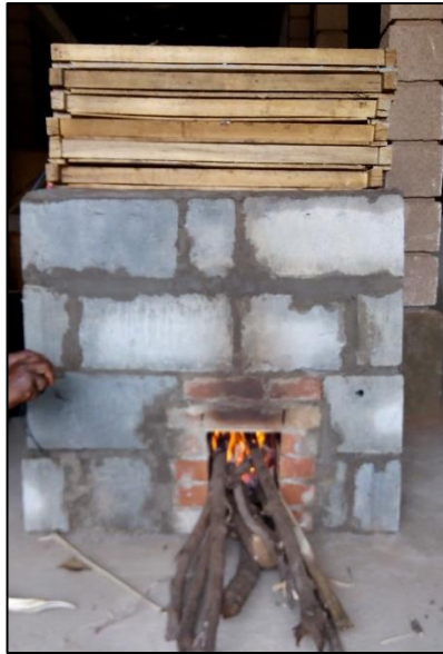
Figure 28 SNV Fish Smoker – Morrison Stove Retrofit View 1
