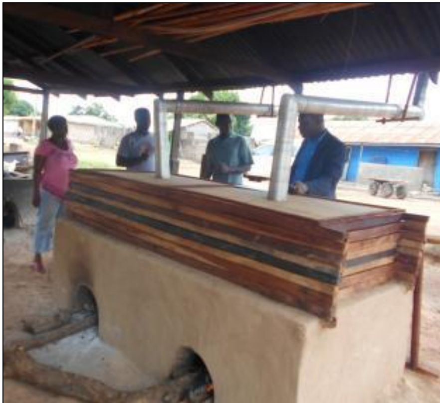
Figure 2 Morrison stove with two work stations
