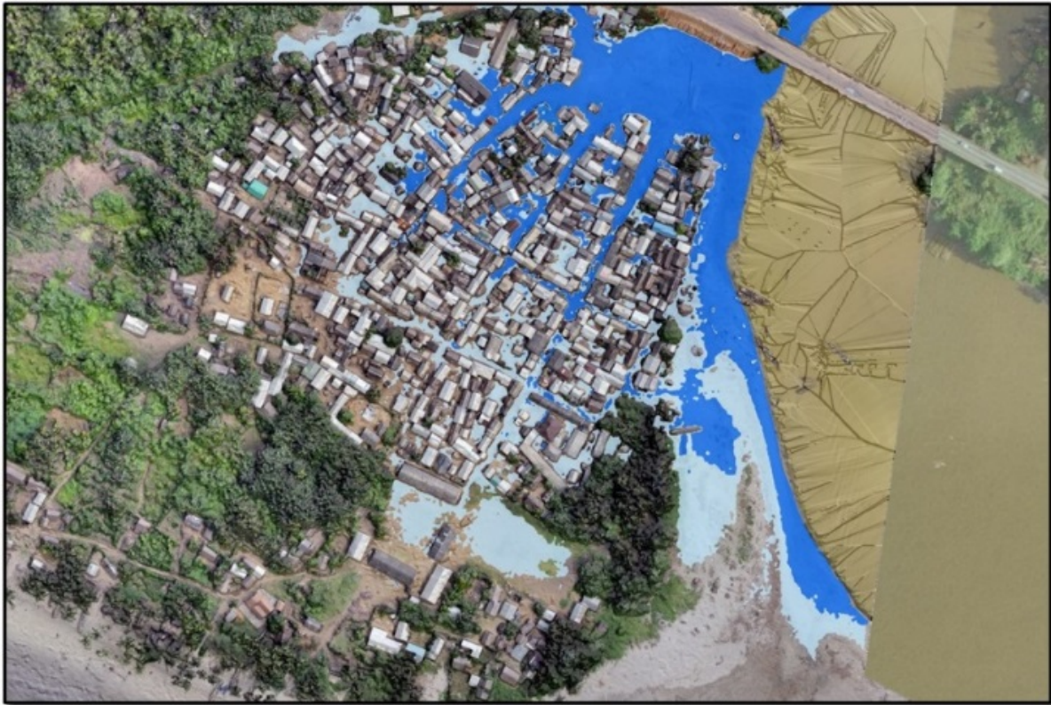
Figure 15: Extent of daily double flooding at the Ankobra estuary
