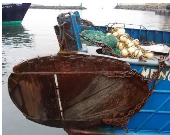
h. trawl door that keeps the spread open on the bottom
