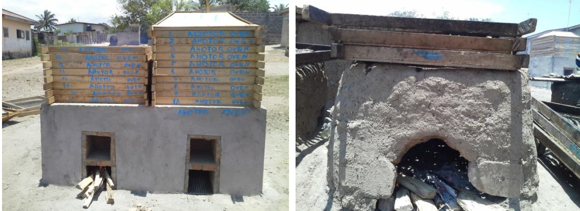
Figure 1 Photographs of Ahotor Oven and Traditional Chorkor Stove
