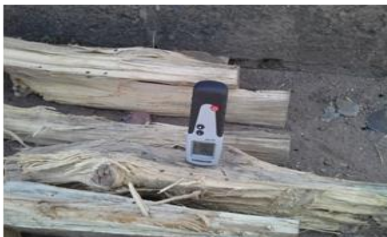
Figure 3 Measurement of wood's moisture content
