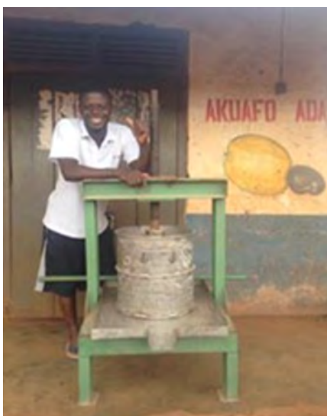
The simple screw press was acquired from MOFA and will allow for processing of the cashew apples.
