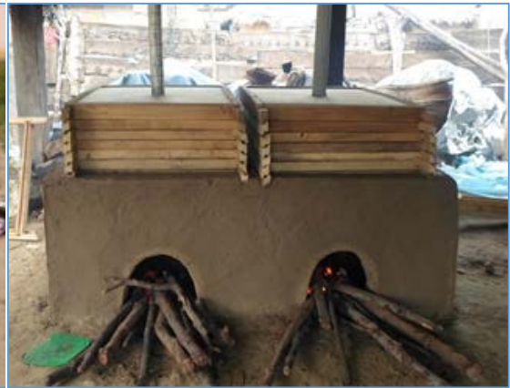
Figure 24 The improved Morrison stove adds a number of energy efficient features
