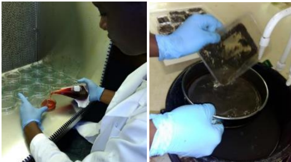
Figure 18: Inoculation of samples for microbial load determination (left). Washing sediments for particle size analysis (right)
