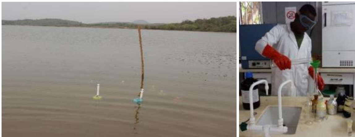
Figure 24: Field experimental setup for nutrient flux determination at Sumina Lagoon (left). Student preparing reagent for laboratory analysis of samples (right)
